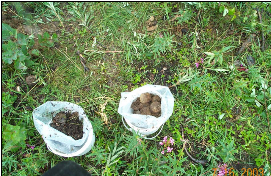
a. Thirty-increment sample from a 2-m × 6-m area at FP Sally divided into the surface 1 cm and the top 1 cm of the underlying mineral soil.
