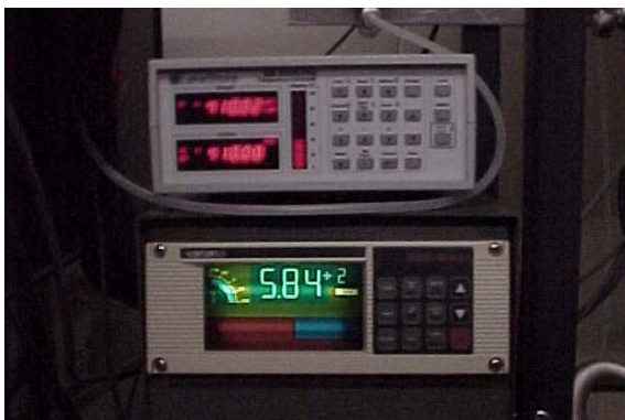
Figure 59. Photo of the Varian the Multi-Gauge controller.
