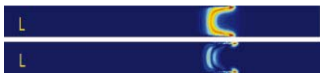
FIG. 10. (Color) Mean (top) and standard deviation (bottom) of the labeled protein concentration L at t = 0.50 s. The initially at profiles are now severely distorted. The values of the contour levels go linearly from 0 (blue) to 3.2 \times 10^{-4} mol/l (red) in the top plot and from 0 (blue) to 10^{-4} mol/l (red) in the bottom plot.
