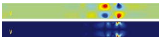
FIG. 15. (Color) Mean (top) and standard deviation (bottom) of the wall-normal velocity at t = 0.50 s. The mean of this velocity has a magnitude of up to 6% of the initial streamwise velocity. The values of the contour levels go linearly from -0.56 mm/s (blue) to 0.56 mm/s (red) in the top plot and from 0 (blue) to 0.26 mm/s (red) in the bottom plot.
