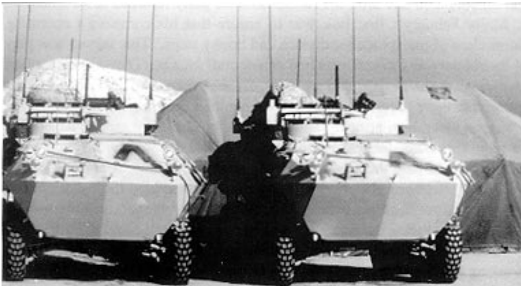
Two command and control variants of the light armored vehicle (LAV-C2) appear outside a command post in northeastern Saudi Arabia during Operation Desert Storm. The LAV-C2 was used as a mobile command post by LtGen Boomer and his subordinate division commanders during the war.
