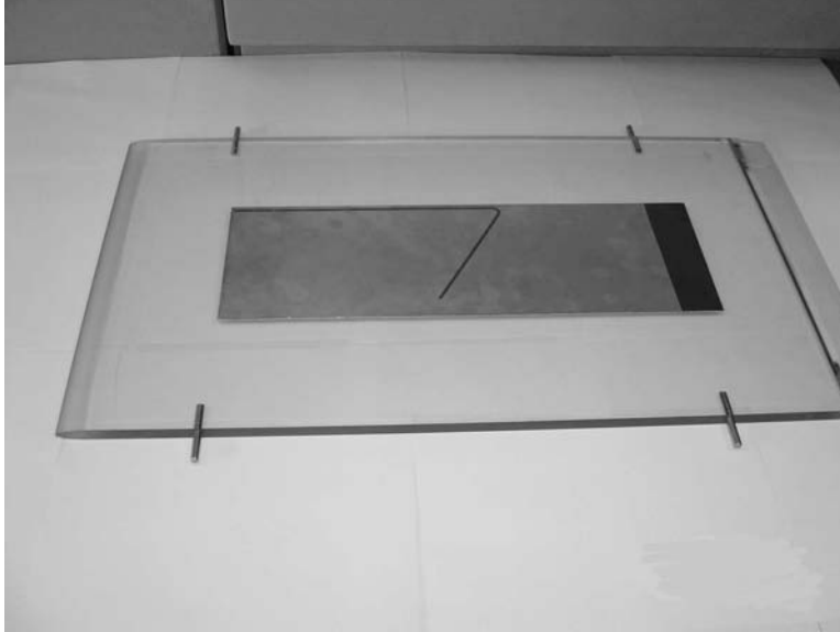
Figure 3.3: Center plate used to support the electrode.
