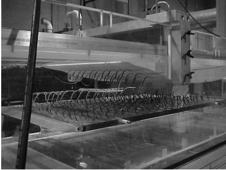
Figure 3.5: Use of mylar strips as tufts.
