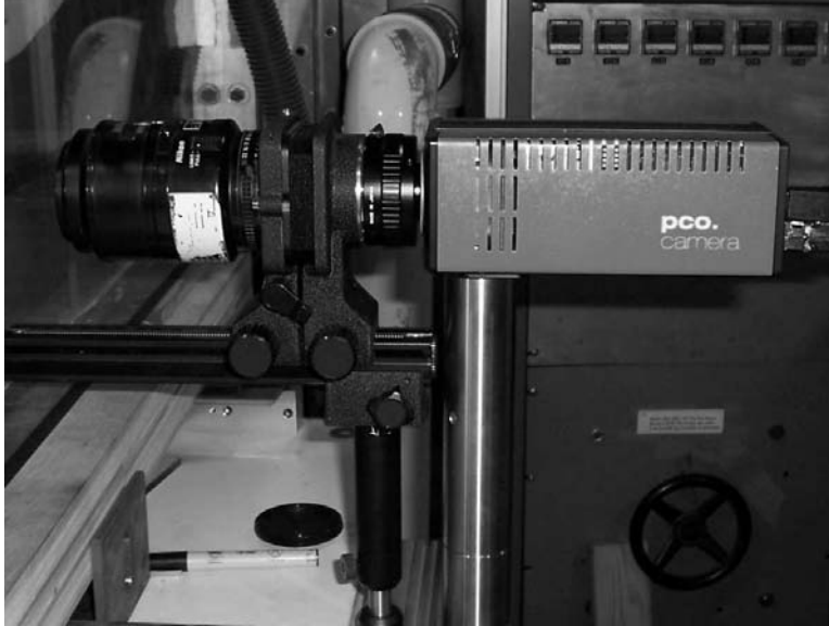
Figure 3.16: High speed digital camera used with PIV.
