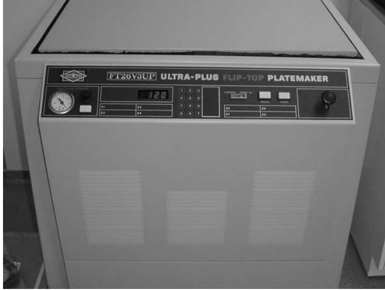
Figure 3.9: UV Exposure Unit with 3000W Metal Halide Bulb.
