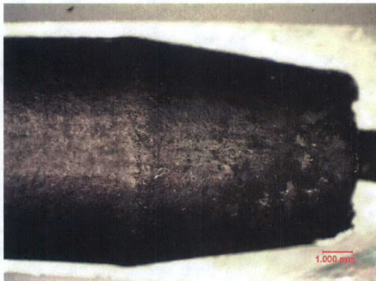
Figure 26 Sectioned view of localized case wall necking observed
