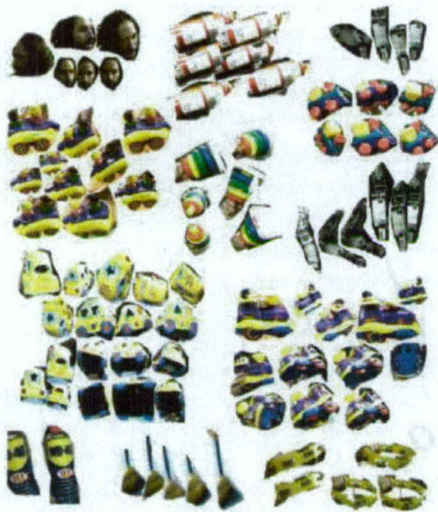
Fig. 14. Sample of objects segmented from oscillatory motions, under different views. Several segmentations of the robot's arm (and upper arm) are also shown, obtained from rhythmic motions of robot's arm (and upper arm, respectively) in front of a mirror. Shown are sample segmentations from a large corpus consisting of tens of thousands of segmentations computed by the real-time segmentation algorithm.
