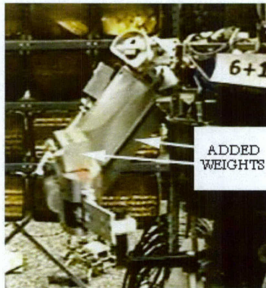
Figure 4-23: REAL To demonstrate robustness of the oscillator system, it was used with two 1 Kg masses attached to the upper and lower parts of the arm. These masses effectively double the inertia of the arm links. Their effect on the oscillator control was to make the system turn the crank slower, but did not disrupt the crank motion. In this picture all six degrees of freedom of the arm were used to turn the crank.
