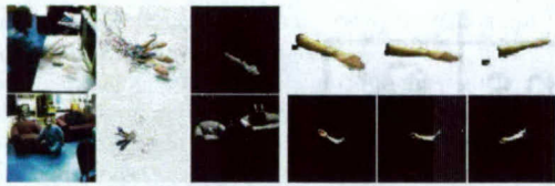
Figure 5. Human waving the arm to facilitate object segmentation. Upper row shows a sequence for which the skin-tone detector performs reasonably well under light saturation. Lower row shows background sofas with skin-like colors. The arm's reference size was manually measured as 5.83 pixels, while the estimated value was 5.70 pixels with standard deviation of 0.95 pixels.
