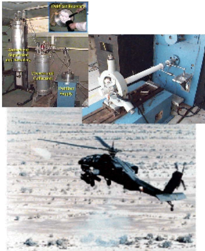
Figure II-18. Left: Anti-Solvent Process. Right: No-Lead 2.75" Missile on Test Stand. Bottom: Helicopter Firing 2.75" Rocket.
