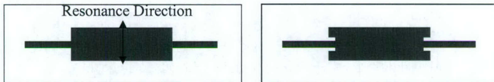
Figure 1.8: Left – Resonator connected along its width dimension showing resonance direction of interest; Right – Resonator with notched attachments.
