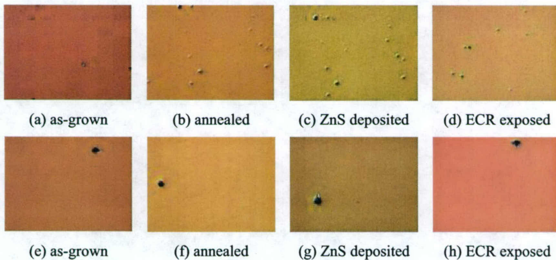
Figure 8. Surface morphology investigations of sample MCT02333c17 following various processes. Images were acquired with x100 magnification for a – d and with x500 magnification for e – h.
