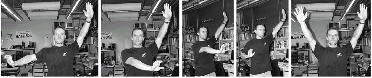
Figure 15: The virtual joystick mode of the GestureDriver , showing right, left, forward reverse, and stop commands [Fong 00].
