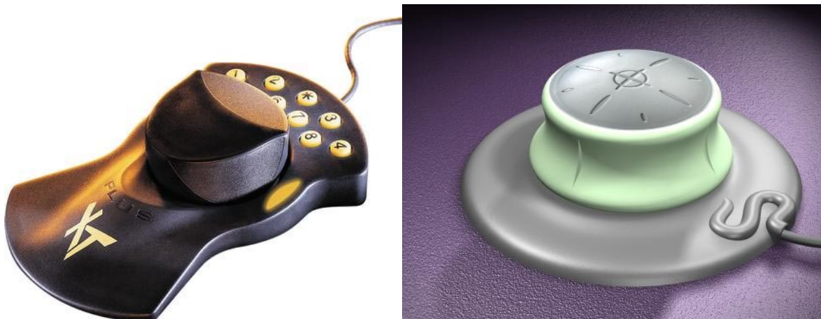
Figure 11: a) Magellan/SPACE MOUSE "Plus XT" (188 x 120 x 44 mm and 720 grams) and b) Cyberpuck (140 x 140 x 45 mm and 510 grams).
