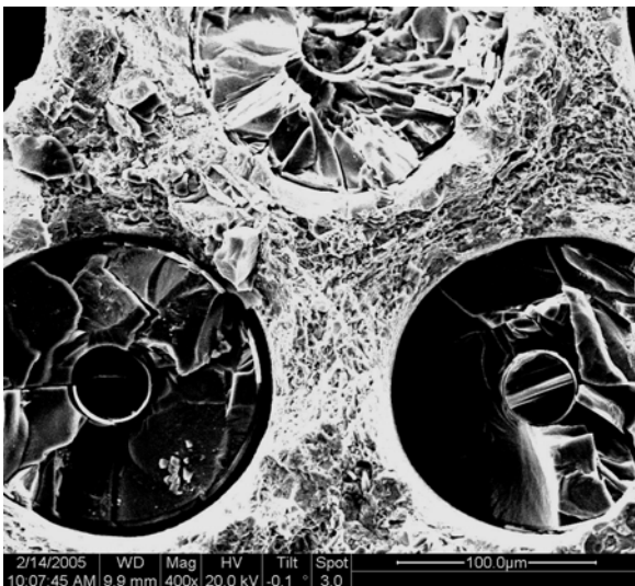
Figure 80: Specimen TMC-04, 1: catastrophic fiber failure
