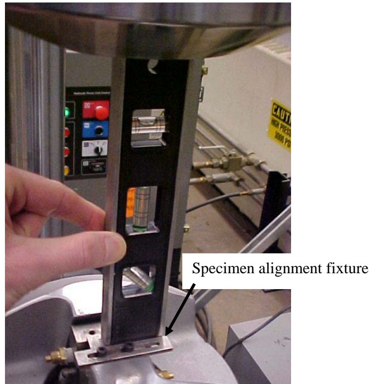
Figure 8: Aligning the specimen alignment fixtures
