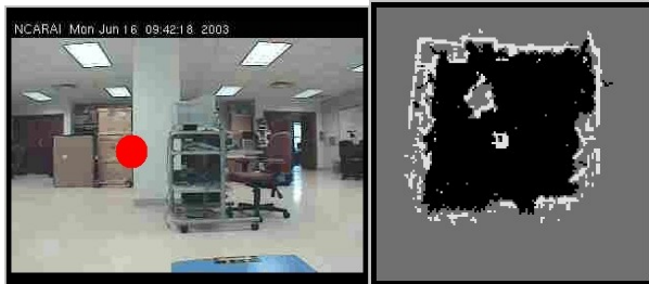
Figure 3. Touch screen display of robot's eye view (left) and mapped representation (right) of environment. (The large (red) dot on the pillar in the left display indicates where participants touched the screen.)
