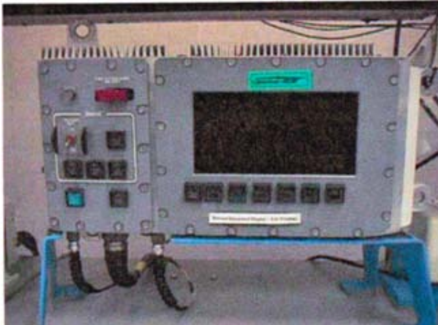
Figure 1. Driver's integrated display with vertical cooling fins on the top wall.
