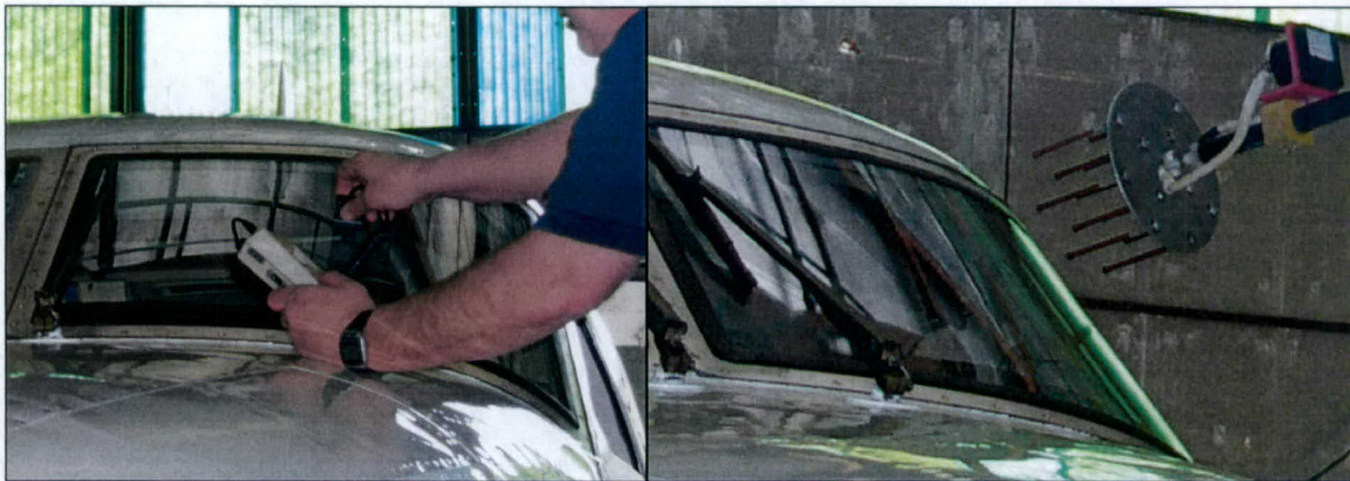
Figure 11. Surface resistivity measurement and charge induction.
