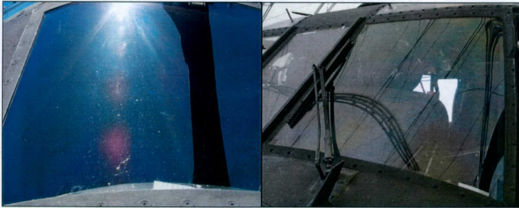
Figure 9. Pitting on unprotected windscreen (left) and no damage on protected windscreen upon removal of the MTOWF (right).
