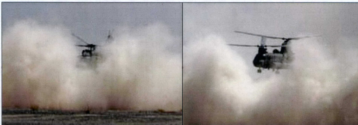
Figure 8. Brown-out durability testing for UH-60 (left) and CH-47 (right).
