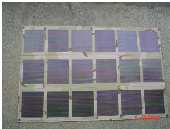
Figure 6. Global Solar P-4 Array (From: Atira Technologies)
