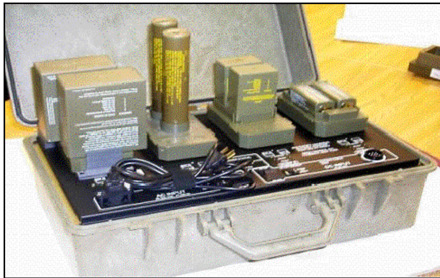
Figure 21. PP-8498/U Multi-Port Universal Battery Charger 87
