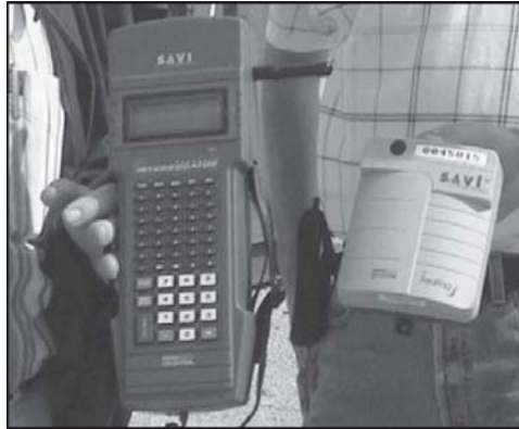
Figure 6. Portable RFID reader and active RFID tag (From: AFLMA)
