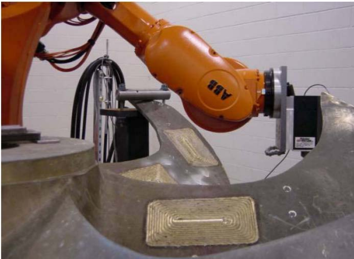
Figure 4. Area Processing of a Marine Propeller (From 14). The robotic machine from NSW Carderock is used to manufacture propeller. A spiral pattern is shown on the propeller.
