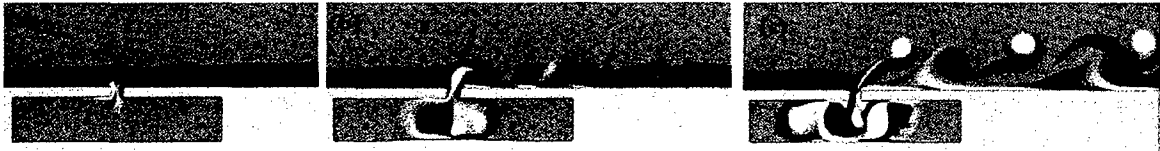
Figure 7-1: Spanwise vorticity plots for three cases where the jet Reynolds number Re is increased. A) Re = 63 . B) Re = 125 . C) Re = 250 . With Re_\delta = 254 , h/d = 1 , and S = 10 . (Reproduced with permission from Rampugoon 2001).
