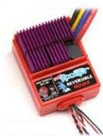
Figure 13. Novak Super Rooster Electronic Speed Control [After Ref[7]
