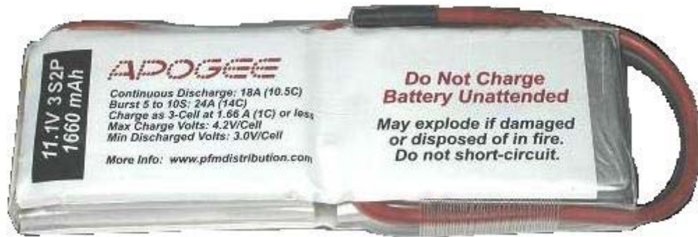
Figure 15. Apogee Lithium-Polymer battery [After Ref.[8]]
