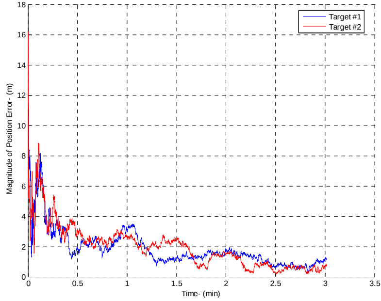
Figure IV-7 The MTT algorithm position error for a normal-case scenario. The plot is done for two targets.
