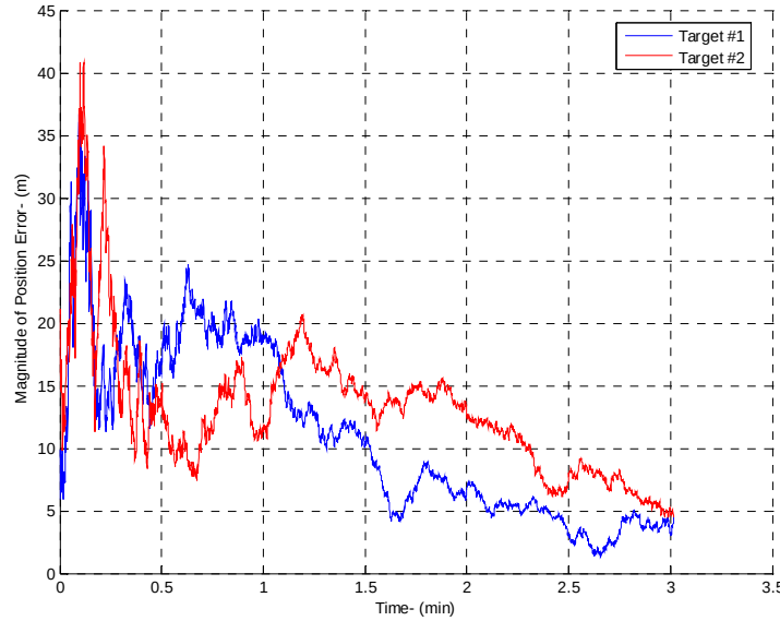
Figure IV-9 MTT algorithm target position error when both targets use reduced RCS coating.
