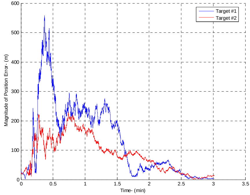
Figure IV-10 MTT algorithm position error, when the combined attack is used.
