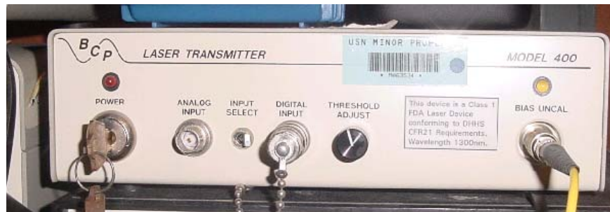
Figure 5. BCP 400 Laser Used as Input to Splitter
