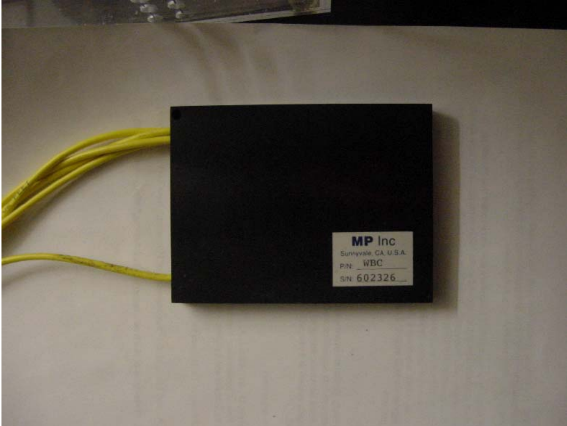
Figure 6. A 1x4 Optical Splitter
