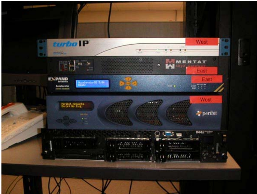
Figure 8. PEP Size Comparison to a 2U Dell Server
