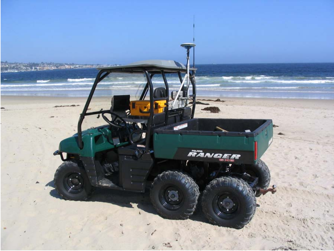
Figure 5. Polaris all-terrain vehicle (ATV) with kinematic GPS (KGPS) and KVH tilt sensor hard mounted.
