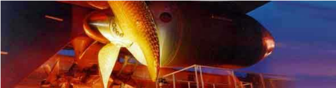
Figure 3. ALSTOM 20MW Azimuth Pod (Mermaid™) [From Ref. 4.]
