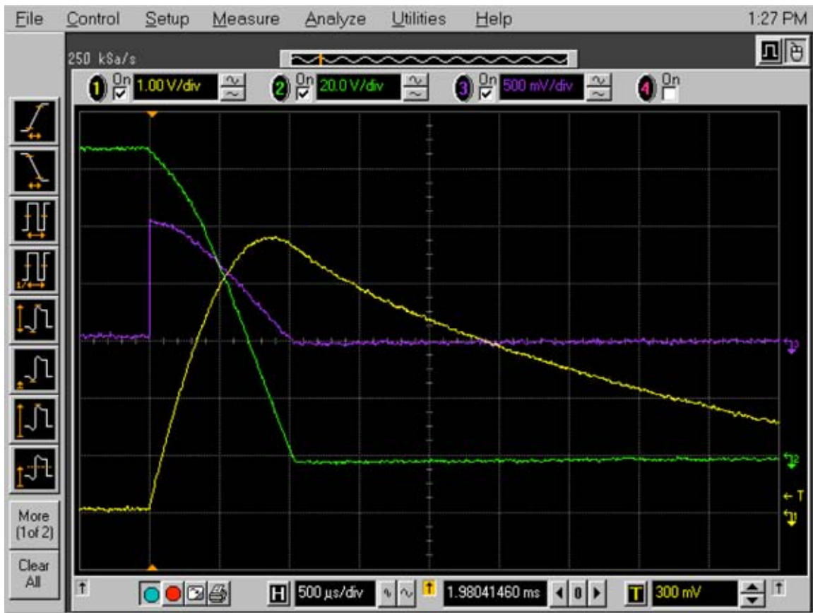
Figure 18. CP Switch Failure-to-Open: Oscilloscope Screenshot. See Table 3 for Parameters
