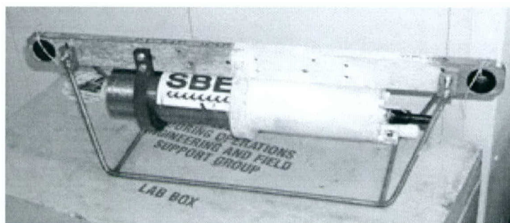
Figure 3: An SBE-16 (SeaCat) painted with white anti-foulant
