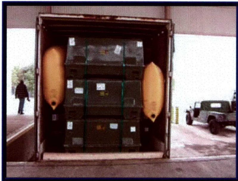
Photo 6. Movement of Passenger Side Air Bag.
