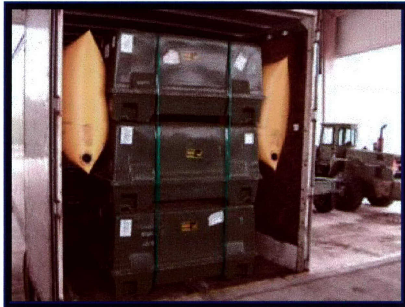
Photo 1. Air Bags Securing the JDAM CNU-589 Containers
