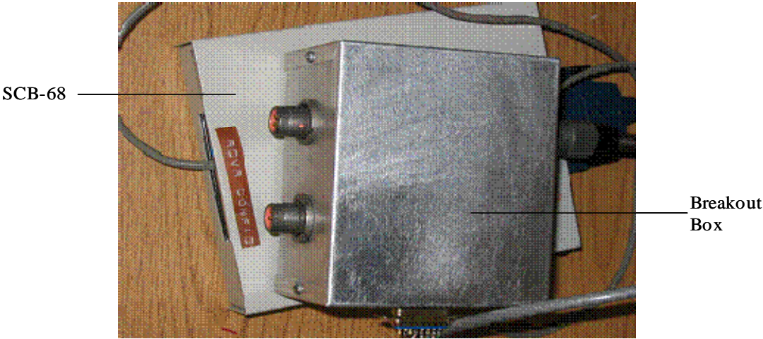
Figure 16. SCB-68 and Break-Out Box
