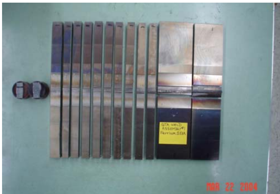
Figure 82 Photograph of Weld Assembly # 1 (Root Side) after sawing specimen blanks and flattening; two metallographic mounts of cross-sections.
