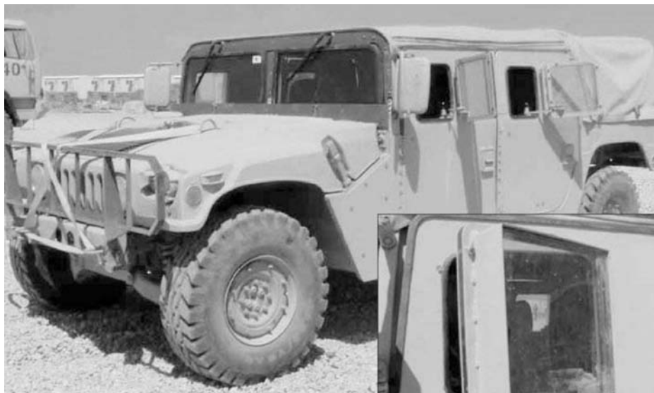
Figure 26: Add-on-Armor Kit Mounted on HMMWV
