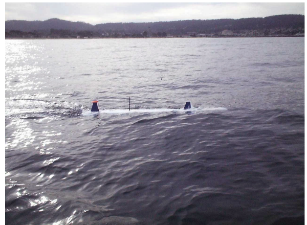
Figure 1. The NPS ARIES AUV in a GPS Pop-up Maneuver (December 2000)
