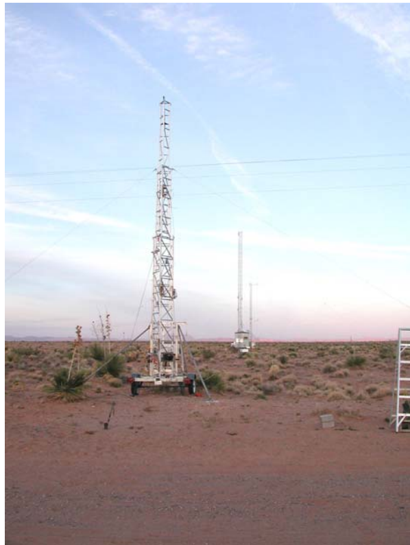
Figure 3.2. The three-tower system used to characterize and quantify the dust emissions from the test vehicles.
