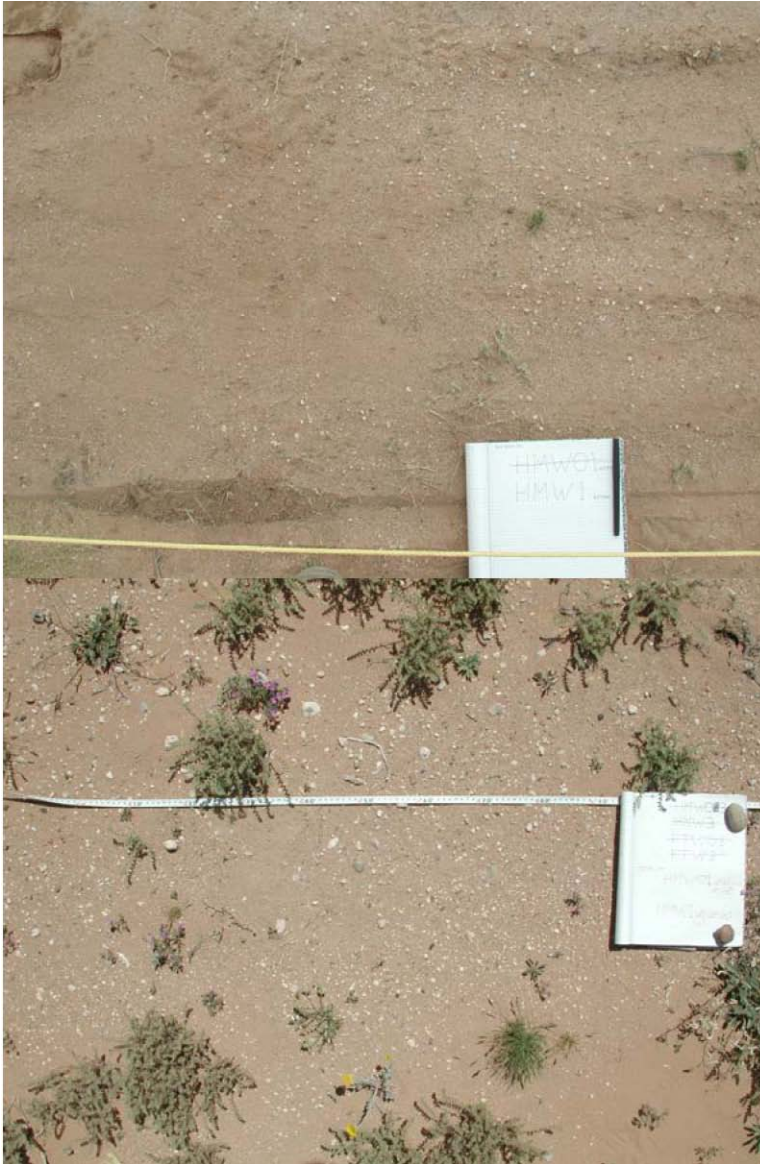
Figure 4.26. Image of the same disturbance plot (Humvee, least disturbed) showing that visual signs of disturbance from vehicle tires are not evident in two years passage of time.
