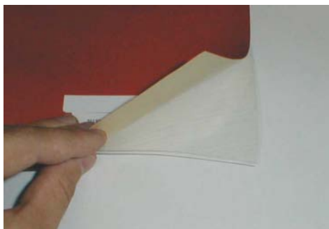
Figure 3. Bladder materials. The clear material is the inner water containing polyurethane, while the outer material is a multilayer laminate barrier.
