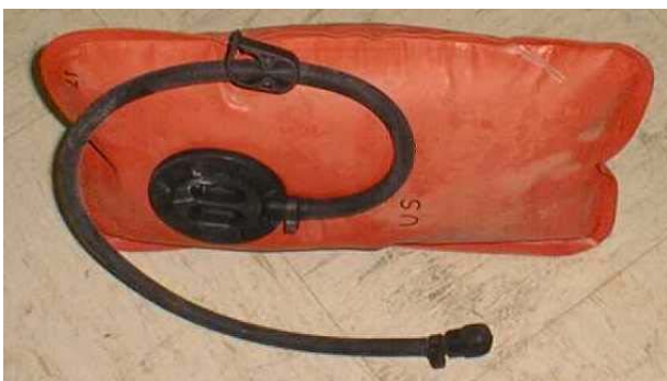
Figure 7. Frozen, filled water pouch. No damage occurred.
