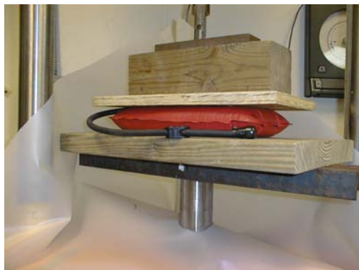
Figure 5. Crush test. In this configuration, the water pouch withstood a load of 1000 lbs with no damage.
