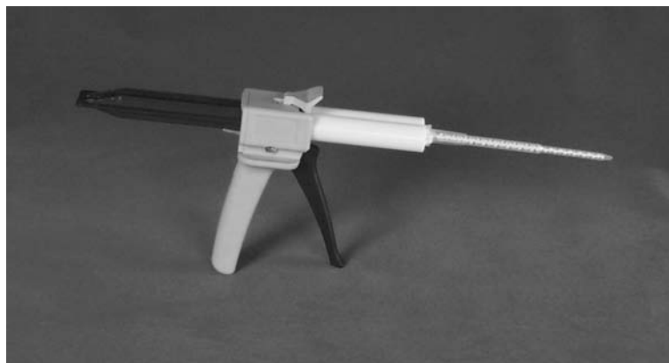
Figure 1. Apparatus for mixing enzymes in aqueous buffer and prepolymer.
