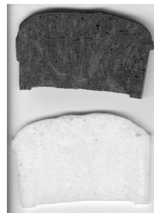
Figure 2. Top sponge, activated carbon incorporated during synthesis; bottom sponge, immobilized AChE sponge.
