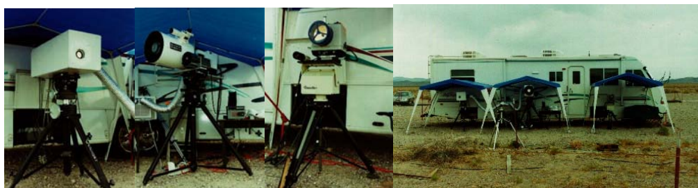
Figure 2. Three Sensors Tested – top from left to right, AIRIS, HISPEC, and TurboFT. Far right shows the three sensors as positioned next to the motorhome during the tests.
