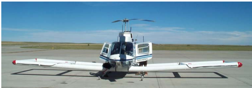
Figure 16. Lobed 3 m X 3 m transmitter configuration. Note the transmitter cable does not extend across a portion of the front boom.
