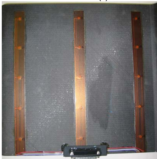
(c) Piezoceramic sensor encapsulated in SMART Layer and mounted on CFRP test structure
