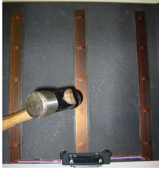
Figure 3: Hammer (2 lbm) used for impacting on sensor to induce sensor damage
