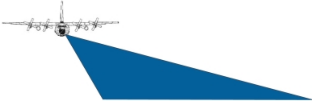
Figure 14. Radar Beam in Elevation and Azimuth when Antennas are mounted in the Pod
