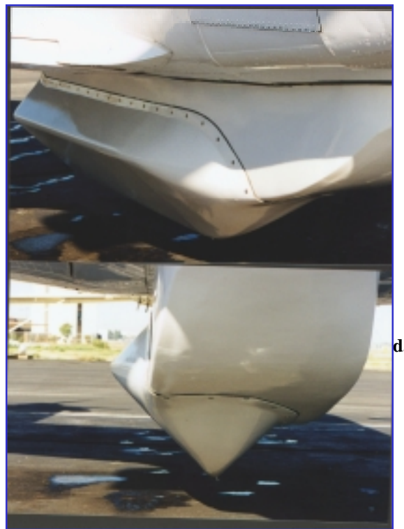
Figure 12. Horn Antenna Installation on a C-12 Baggage Pod
