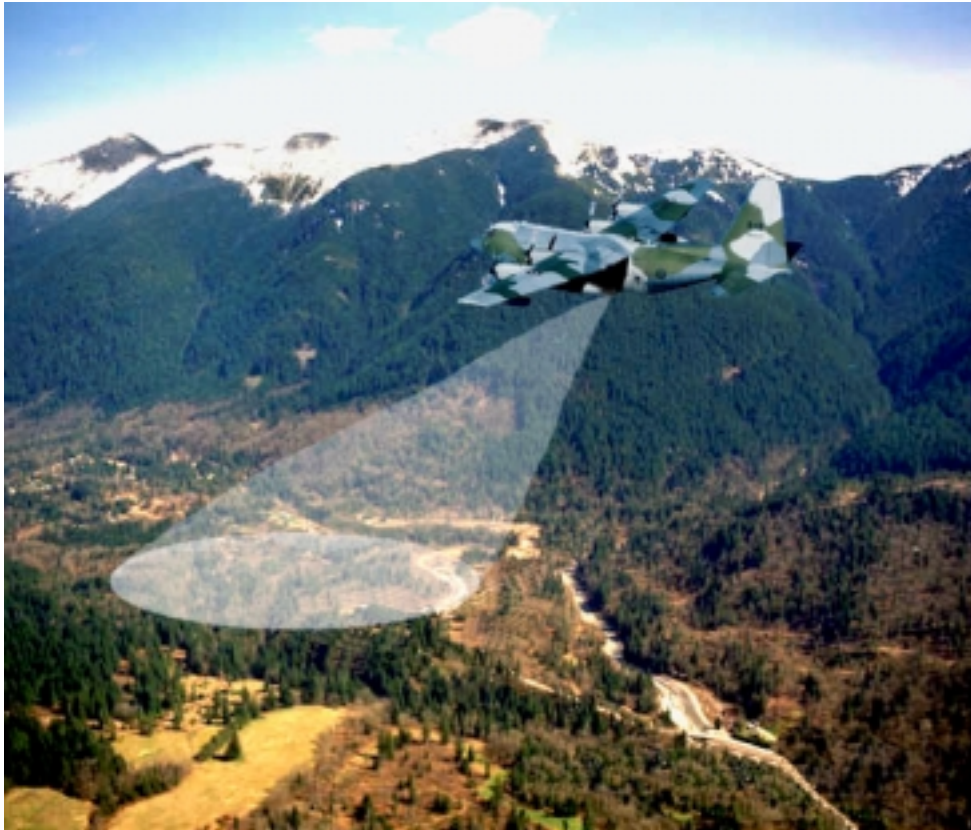
Figure 16. A CC-130 Showing the Radar Beam in relation to the Aircraft Structure
