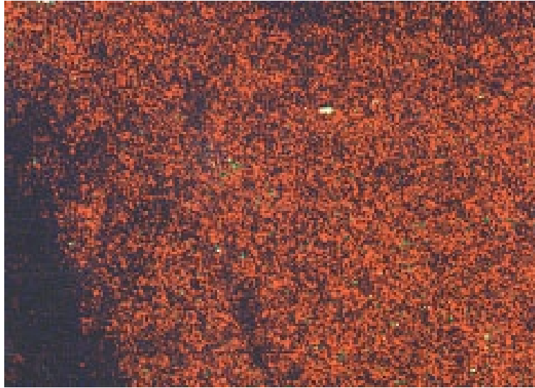
Figure 7. An Example of a Metal Plate Target (broadside) 2x5m under Tropical Forest Signal to clutter ratio is + 20dB
