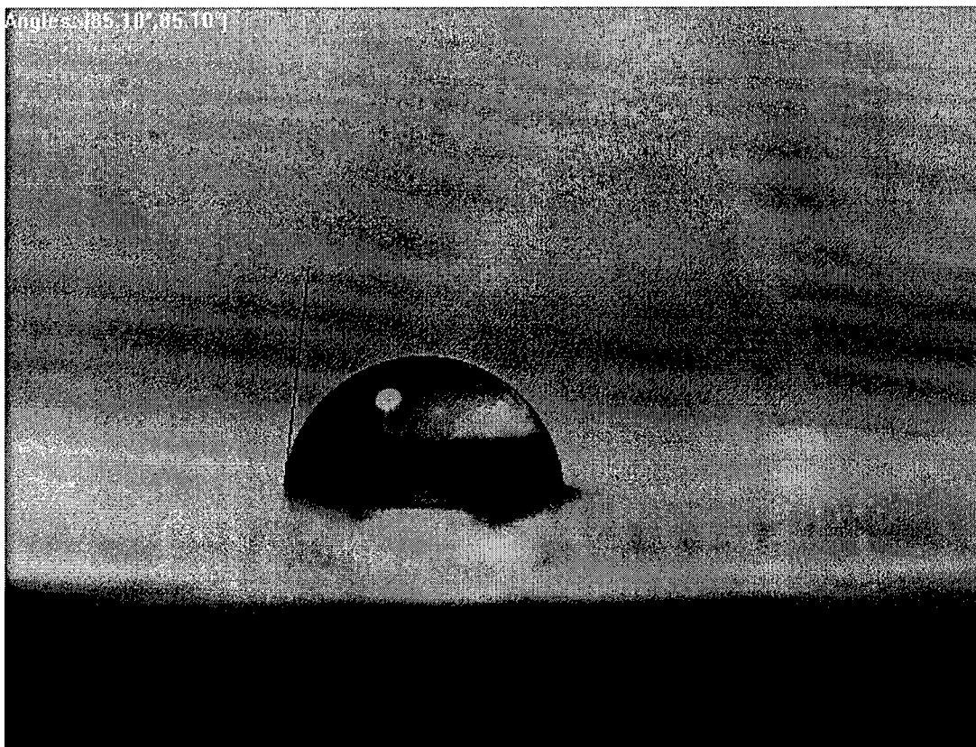
Contact Angle – EMI BF4 on Teflon – 85.1 degree
