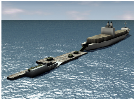
Figure 1. Roll-On Roll-Off Discharge Facility
