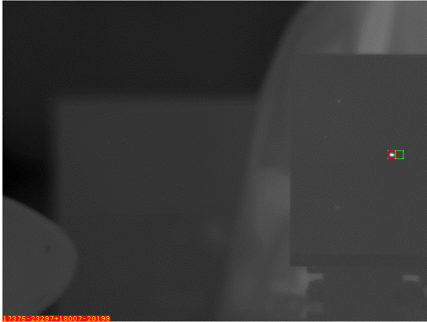
Figure 8 Point target, 0.17 mrad diameter, to the right and with coma distortion
