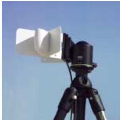
Figure 10. Horizontal orientation of the CORNER249 (Vertical polarization)
