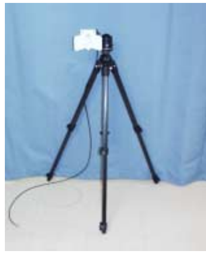
Figure 4. Cirronet 9 dB corner reflector antenna
