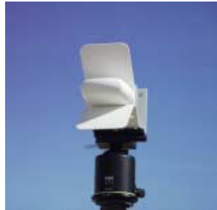
Figure 11. Vertical orientation of the CORNER249 (Horizontal polarization)
