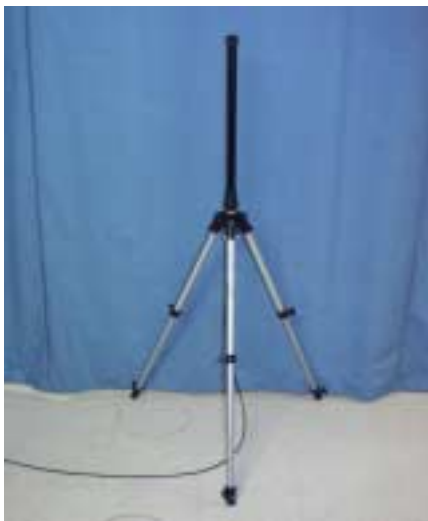
Figure 3. Cirronet 9 dB omnidirectional antenna
