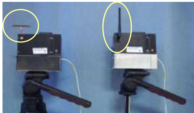
Figure 9. Remote antenna mounting
