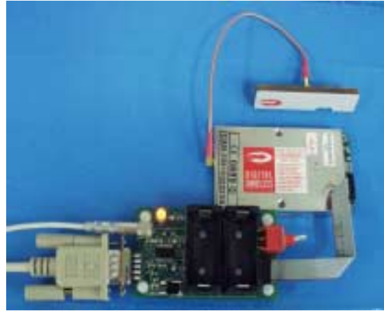
Figure 2. WIT2410 serial port transceiver interface
