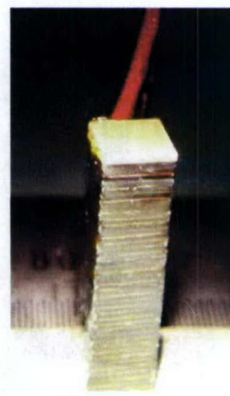
Figure 7. PMN-PT stack actuator.
