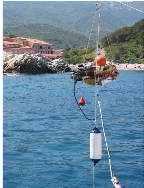
Figure 3: Left, photograph of the burial jig being deployed during a sea-trial in July 2004. It is used to insert four receivers and two projectors into the seabed with a fixed geometry. Right, photograph of the pressure vessel being deployed during a sea-trial in June 2004. It has two isolated internal compartments, one that serves as a junction box for all sensor, power, and communications cables and a second that houses the acquisition system and electronics.
