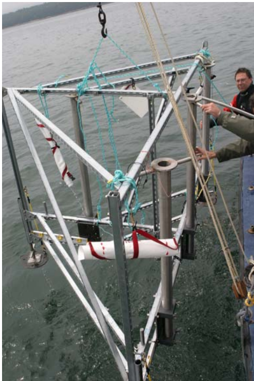
Figure 3: Left, photograph of the burial jig being deployed during a sea-trial in July 2004. It is used to insert four receivers and two projectors into the seabed with a fixed geometry. Right, photograph of the pressure vessel being deployed during a sea-trial in June 2004. It has two isolated internal compartments, one that serves as a junction box for all sensor, power, and communications cables and a second that houses the acquisition system and electronics.
