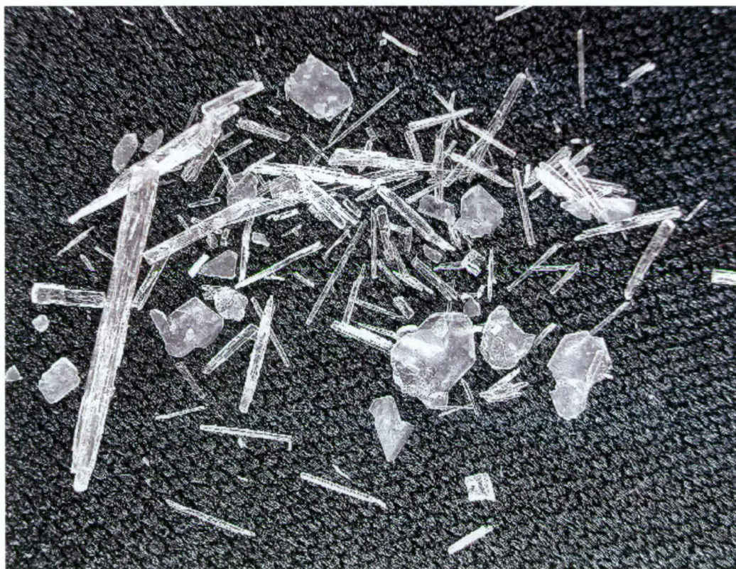
Photo 6.1 Synthesized DIPU By Addition of DICDI to Water
