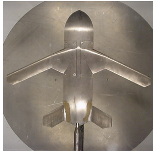
Figure 10: Completed strike tanker mounted in wind tunnel.
