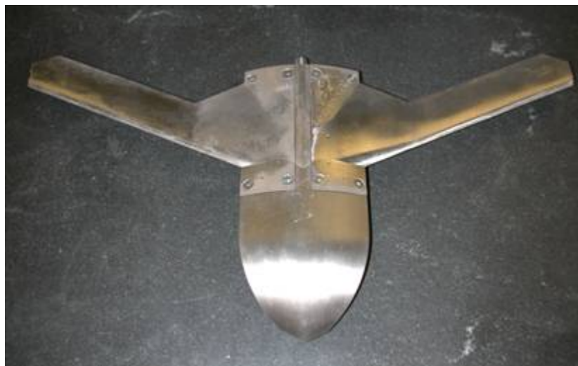
Figure 5: Wings and forward fuselage assembly after polishing process (28).
