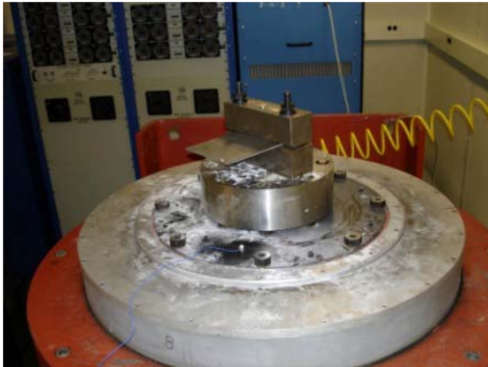
Figure 19. Initial Test Setup with Old Base Plate
